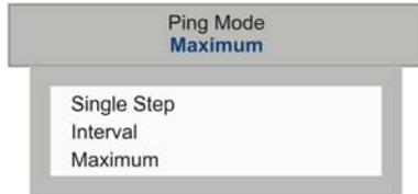
This will make the ES70 ping with maximum speed. The time between each ping is automatically determined by the current depth and pulse duration.
