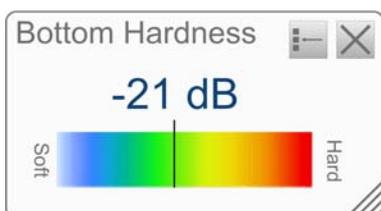
The vertical line in the hardness colour scale positions the current ping. The hardness of the current ping is also shown with the numerical value.
